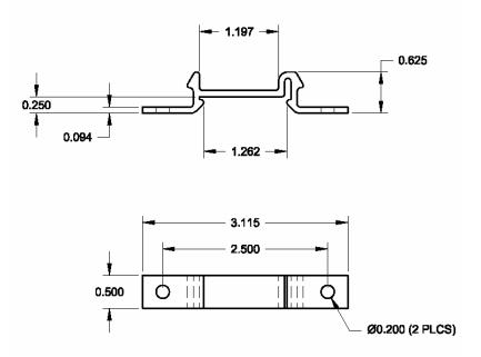
Figure 2: Mounting Clip Dimensions (units are inches)
